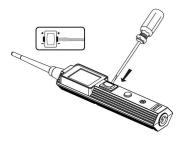
② Make sure to install the switch straight and press until flush with casing
