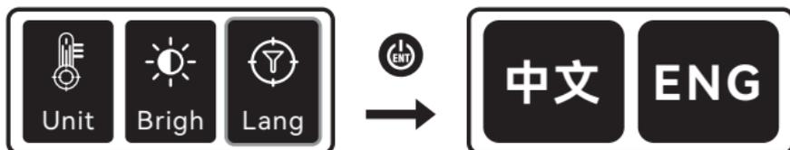
Use the **Toggle button** to switch between different languages, and press the **Enter button** to select and save the language. Once the setting is completed, the display will automatically return to the main interface.
