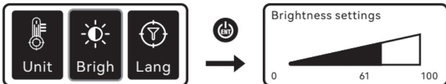
Press the **Enter button** can adjust the backlight, while long-pressing the **Enter button** enables fast adjustment. Once the adjustment is complete, pressing the **Toggle button** will save and exit the brightness, automatically returning to the main interface.
